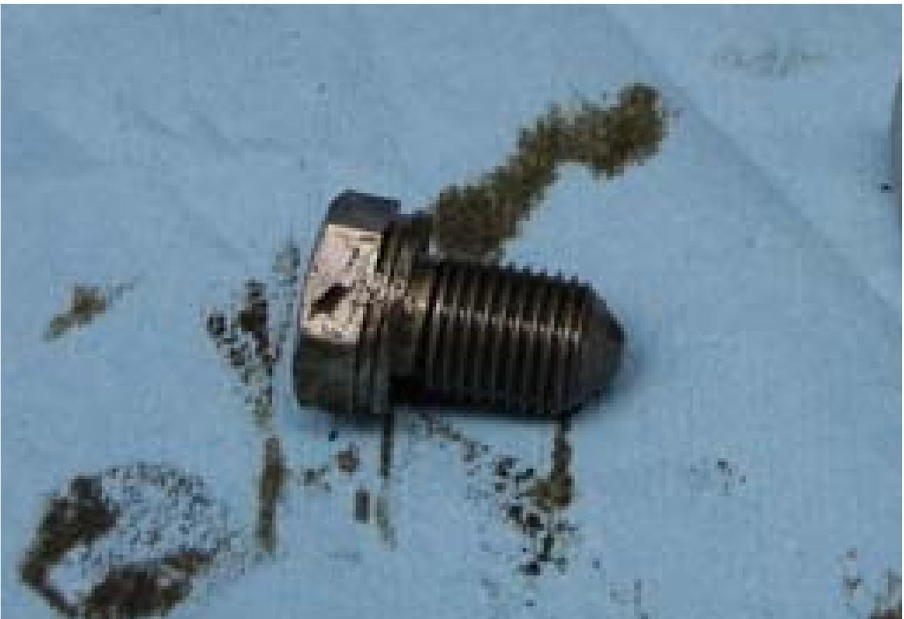
7. Replace the sump plug w/washer with a new one.
