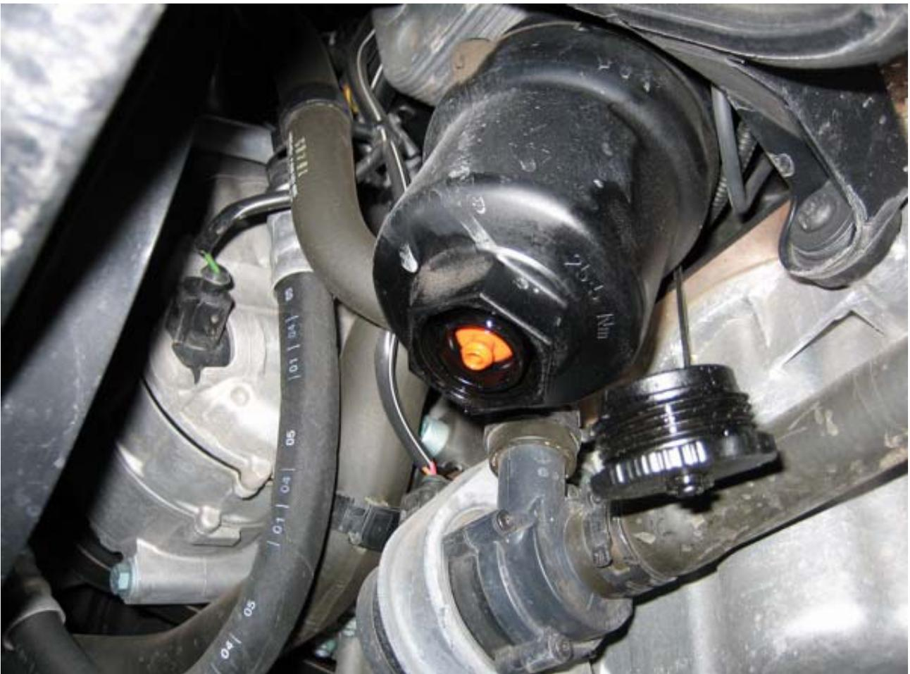
**3. Unscrew the cap cover, (it's tethered to a cable) to expose the orange coloured bleeder valve.**
