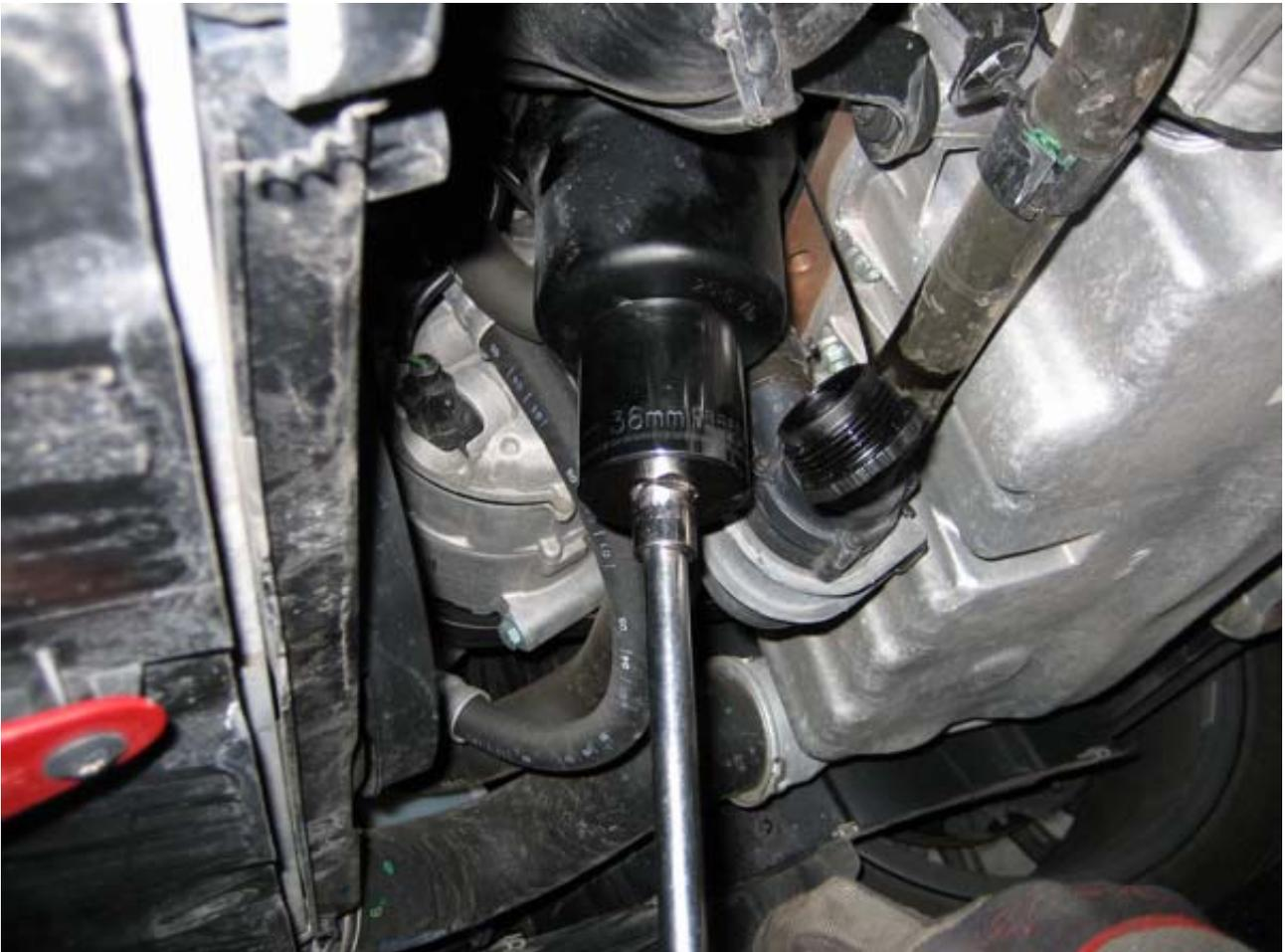
**5. Attach the 36mm socket w/extension bar to a ratchet & remove the lower portion of the oil filter housing. Inside you will find two replaceable items - filter element & o-ring seal, (part no. 06D 115 562) see below.**
