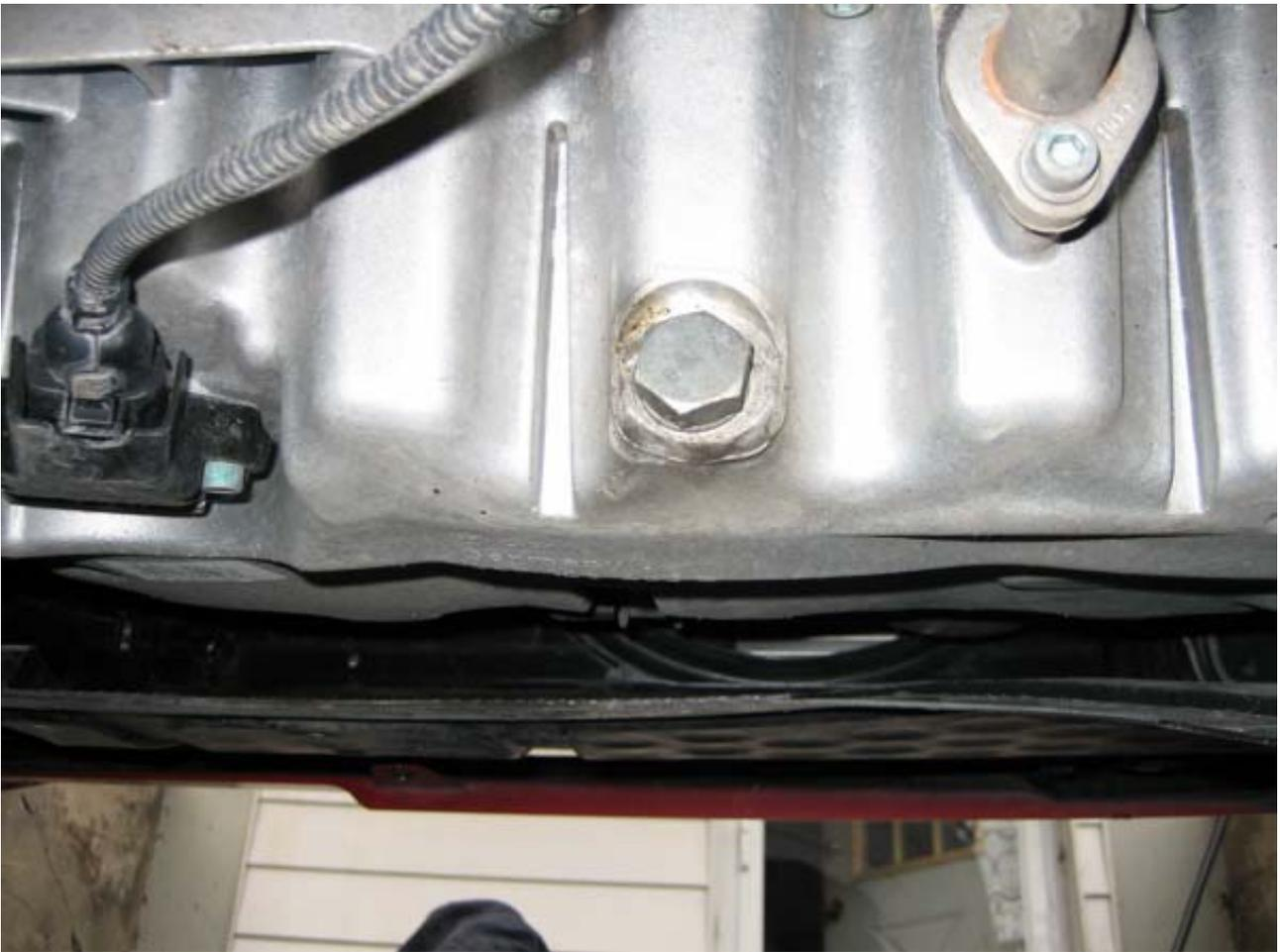
6. Locate the oil drain plug on the back of the oil pan, (facing the rear of the car).
