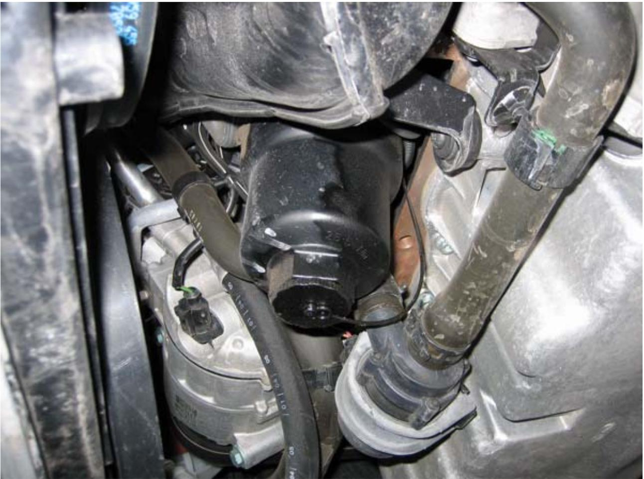
**2. Locate the oil filter housing.**
