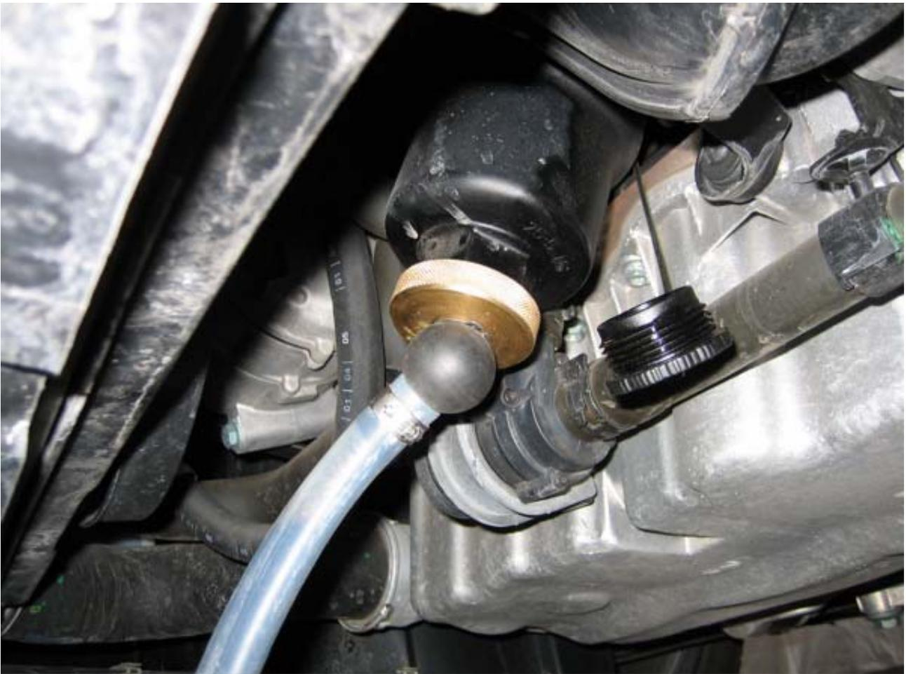
**4. Attach the VW T40057 tool to the bleeder valve by screwing it into the oil filter housing. Allow all the oil in the filter housing to drain out before removing the tool.**
