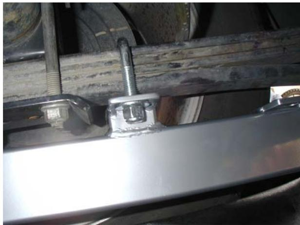
4. Install flat washer, lock nut, onto other side of 'U bolt'.
