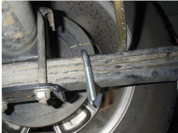
3. Carefully raise the traction bar up to the 'U bolt' in front of the axle (getting someone to lift the front of the traction bar will make this easier) inserting the 'U bolt' through the front (shortest mounting plate) mounting plate holes. Start one nut so traction bar will hang from 'U bolt'. **NOTE: flat washer must be installed on 'U bolt' before lock nut is installed.**
