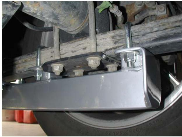
6. Before tightening the nuts make sure the snubber is centered with the spring eye. (It's easier if you have some one else tell you when it's lined up so you can move the bar if needed)
