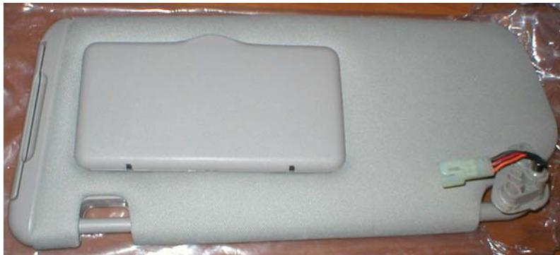
This isn't a problem, we'll just use the two-wire black harness off the OEM visor and attach it to the new HomeLink visor so it will plug back in to the factory harness in the roof.
