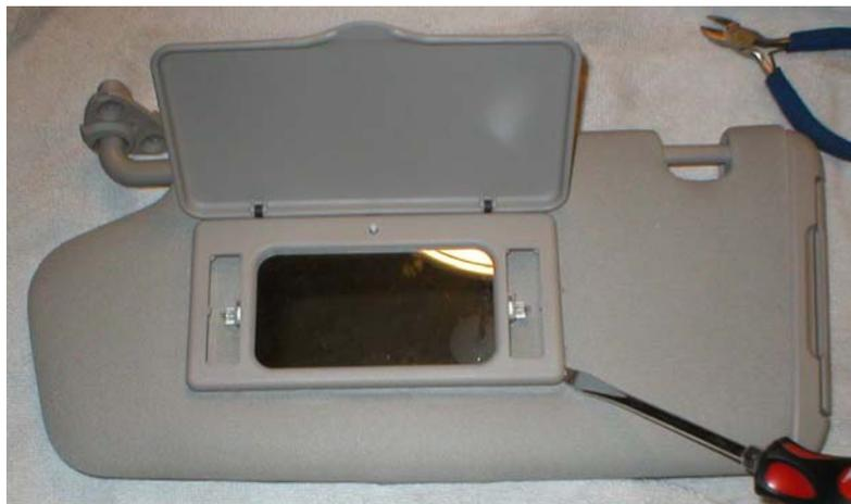
Using the wire cutters, cut the red and black wires to separate them from the visor lights, and then pull the two-wire harness with the black plug on the OEM mirror out of the visor.
