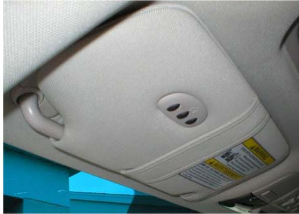
With the ignition "On" or set to "Acc" you can test the vanity Mirror by opening it, lights should come on. Test the HomeLink by pressing any of the buttons, red indicator should light up.
