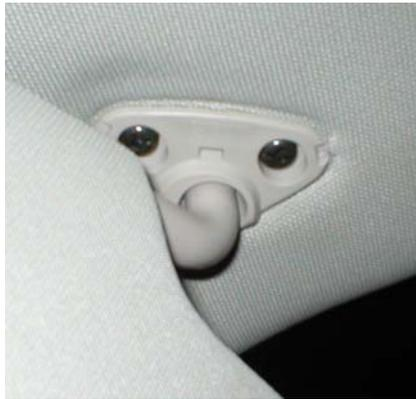
Using the #2 Phillips Screwdriver remove both the screws with one hand while holding the visor in place with the other. Once both the screws are out, gently pull the visor away from the roof. You will see the harness for the lighted vanity mirror, unplug it so you can remove the entire sun visor.
