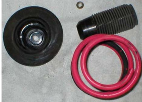
*Start by snapping the USDM dust boot down into position on the Spec B strut:*
