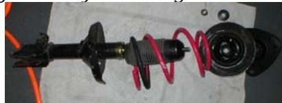
*Out of all those parts you will only need a few things off the USDM front struts to use on the new front Spec B struts. Parts needed are the dust boot, the spring, the top perch and the nut:*
