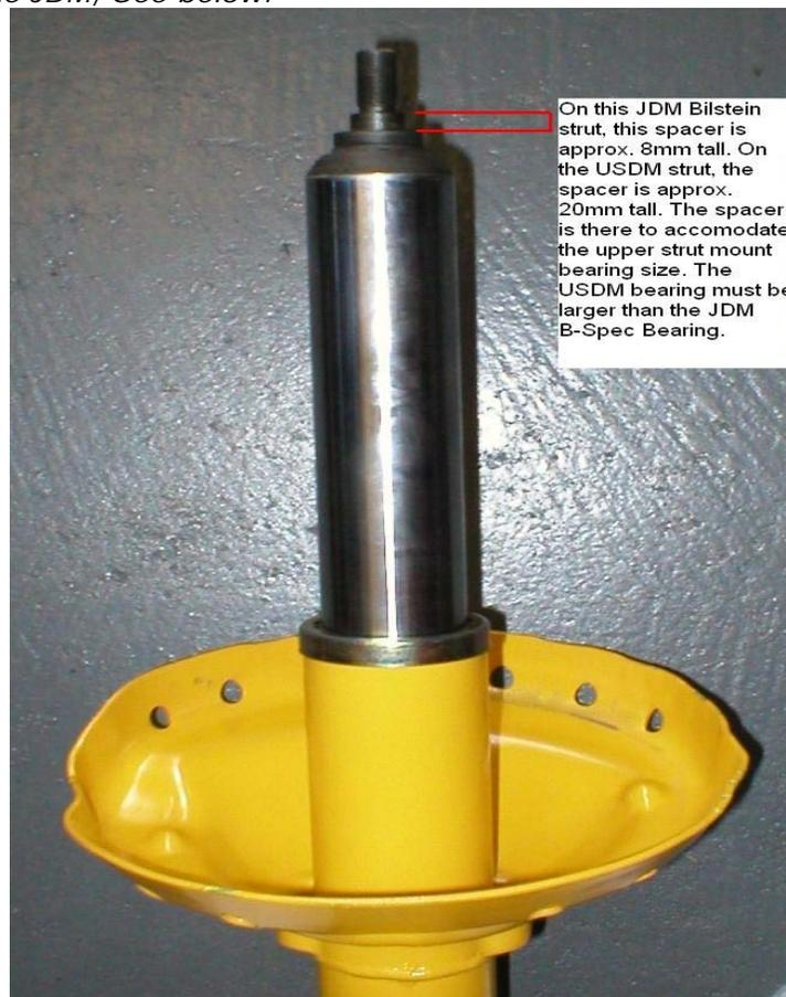
The parts you **WILL** be able to use off the USDM front struts are: the dust boot, the upper spring cushion, the upper perch and the nut to hold it all together. You **WILL NOT** be able to use the USDM bump stop...but that's OK, inverted struts (like these Bilstein's) don't use one.
