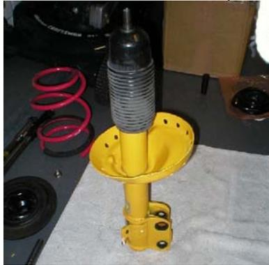
*Then put the spring in place (you will need to use a spring compressor at this point), place the USDM upper spring perch in place (position it properly) with the rubber isolator in place, place the Spec B strut mount in place and secure it all together with the 17mm nut and your all set! Position it in the car and secure all the bolts to the specified torque.*
