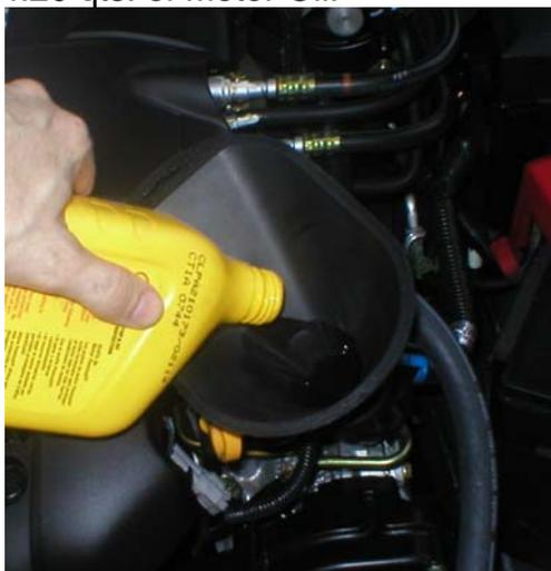
16. Once the engine is full, start the car and let it idle for a few minutes, while idling verify there are no leaks from the oil filter and drain plug.
