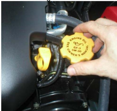
15. Fill Engine with 4.20 qts. of Motor Oil.
