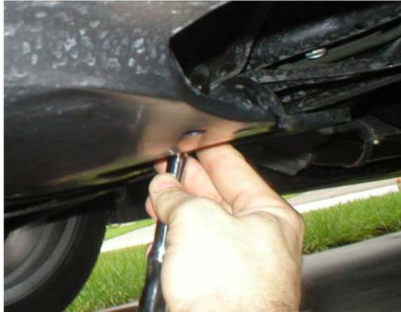
From the side angle (Drivers side) you can see the drain plug a little easier, you can also fit your hand in this hole to remove the bolt by hand once it's loose.
