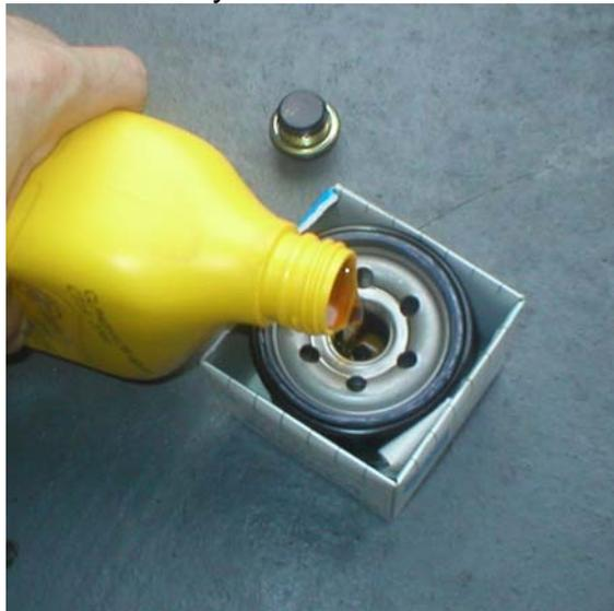
12. Once the filter is full, use your finger to rub a coating of new motor oil on the rubber gasket to ensure a proper seal and reduce the chance of leaks.
