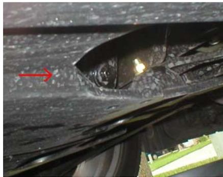
3. Remove drain plug by hand and drain the oil into a suitable pan.
