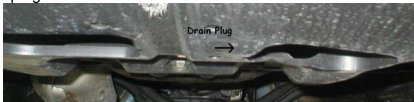
2. Using the 17mm Socket and wrench, loosen the drain plug bolt.
