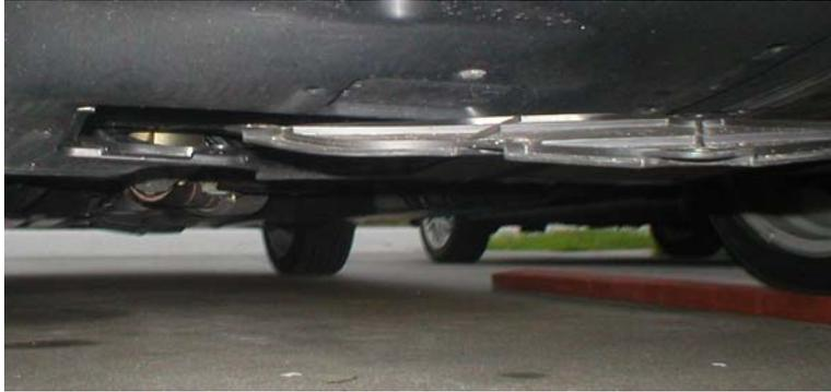
17. Once you have shut the car off you may re-attach the Oil Filter Access panel by moving back into place, inserting the pop-clips and using the #2 Phillips Screwdriver to turn them ½ turn to lock them.
