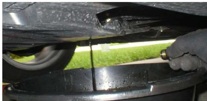
4. Inspect the drain plug and remove the old crush washer, if this is the first oil change the crush washer may be painted onto the plug, just use a small screwdriver to get it free.
